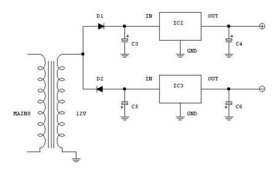
The power supply is very simple. I use mains power, but for portable/remote operations some batteries in series are OK – the OP07 only drains a few mA. In this case omit the regulators; C4 and C6 should be at least 100  $\mu$ F, and mounted close to the op-amp.
